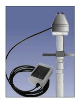
The high temperature PRO Remote capacitance probe features a heavy duty design for use in applications where the temperature exceeds 500°F (260°C). It is used to detect the level of material in a bin, tank or silo or the presence of material in a chute or spout. The probe and the electronics are separated by a cable to distance the electronics from the heat source.
